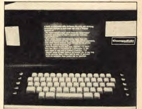
A typical text-editing terminal. No attempt is made to simulate the appearance of the final typeset copy.
